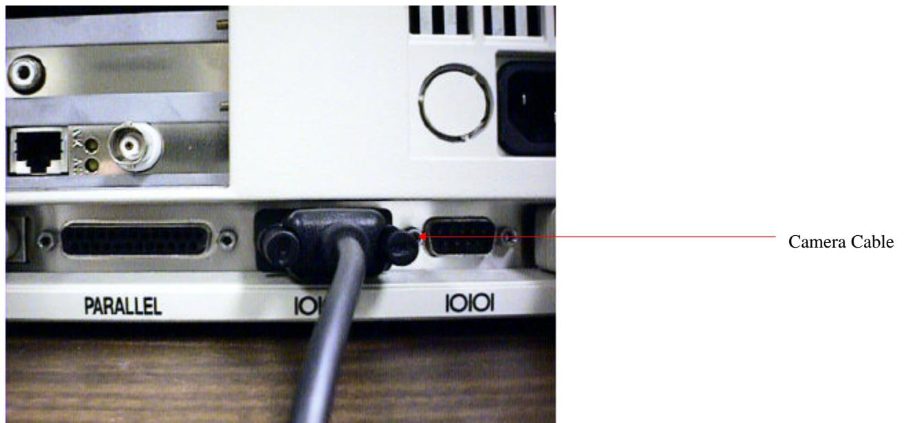
Attached the camera cable to an open 9-pin serial port or, if necessary, detach a 9-pin serial mouse and connect the camera in place of it. (See downloading instructions using Mousekeys or KeyBoard Shortcuts).
