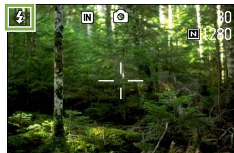
The flash starts recharging. While the flash is charging, the LCD Monitor goes off and the flash lamp blinks. Once charging is complete, the lamp is steadily lit and it is possible to shoot.
